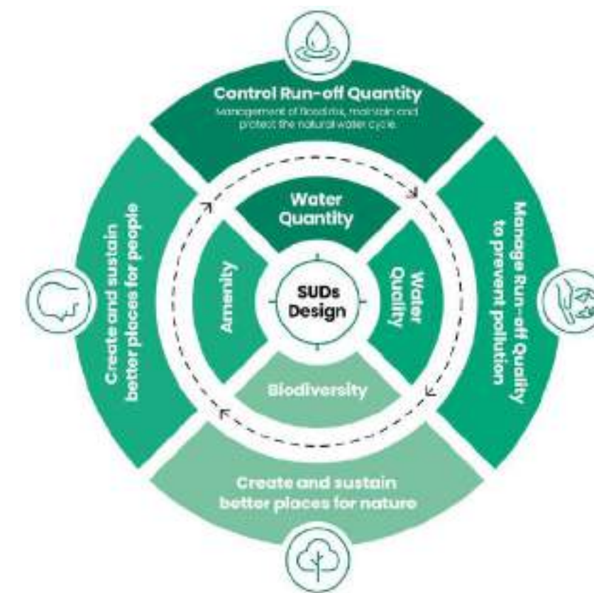
Figure VA.25. Four Pillars of SuDS Design. ©The SuDS Manual C753, Ciria
